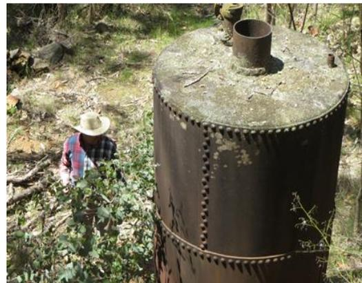
Relic (on right) -12 foot vertical boiler, originally used to power hydraulic sluicing equipment
